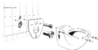
Sound insulation set for wallhung WC Sound reduction: 8–13 dB (A) 156.050.00.1
